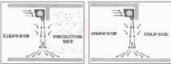
(Interior separation) (Thermal barrier)
